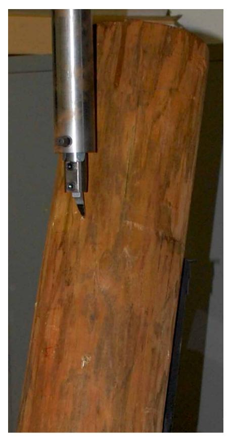
Surface hardness was assessed by means of gaff penetration testing using two different lineman gaffs. One gaff selected for testing was recommended for general pole climbing, while the second gaff was specifically recommended by the supplier for climbing Chromated Copper Arsenate (CCA) treated poles. In addition to gaff penetration testing, surface hardness was measured with a Pilodyn.
